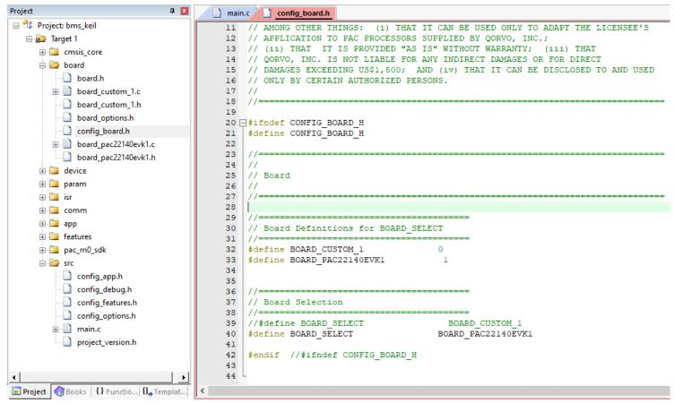
provided to configure the BMS FW. Open the config\_board.h file in board folder and navigate to the "Board Selection" portion of the code. Uncomment the BOARD\_SELECT for the desired PAC EVK and comment out all other BOARD\_SELECT lines. In the example below, the PAC22140EVK1 has been chosen.
