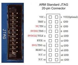
Connect VCC, SWDIO, SWCLK, and a GND using jumper wires to the 4 signals of the PAC EVK 4-pin SWD header labelled [ + SD SCL - ]. This is illustrated in the block diagram on the right.
